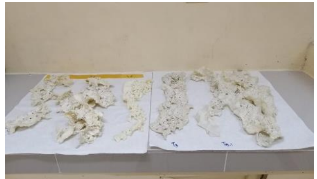
Milled coagulated latex turned into sheets allowed to dry for 7 days for the pre-drying
