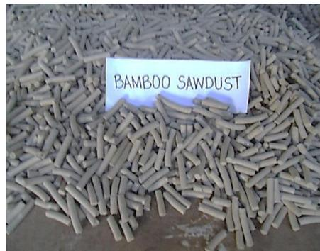
Pellets from bamboo sawdust produced using the FPRDI pelletizing machine.
