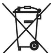
Figure 4: Annex IX to Directive 2012/19/EU provides the symbol that must be printed on the packaging, instructions for use, and warranty of the equipment
